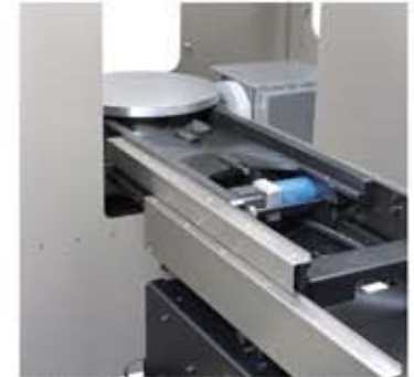
Linear guided pallet delivery system is shown loading pallet onto receiver.
